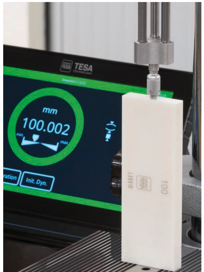
Checking of ceramic gauge block
