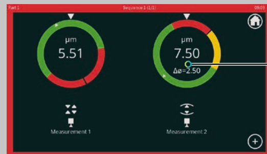
Rotating indicators type display, 2 measurements
