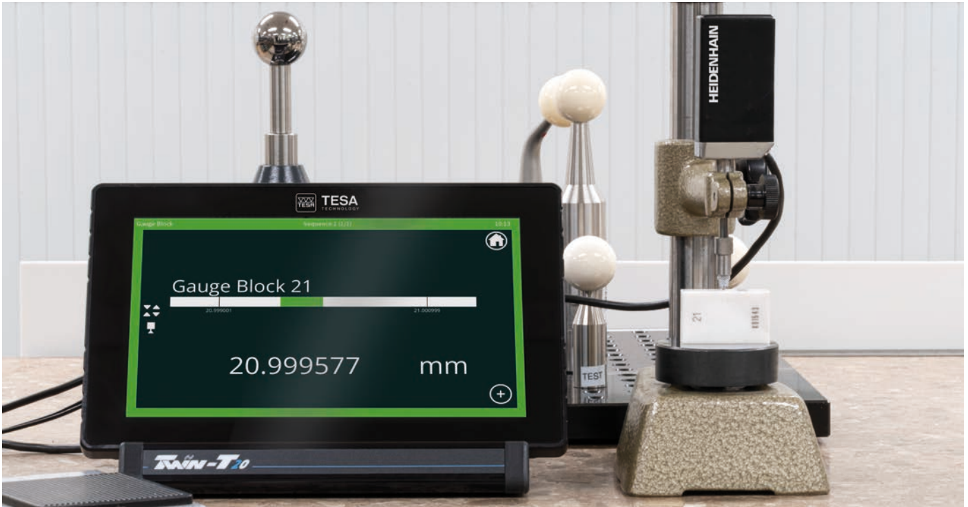
Checking of ceramic gauge block
