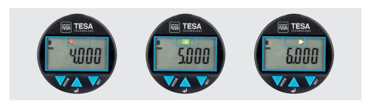
Tolerance mode allows the tolerance indicator to be displayed according to the measurement result. A change in the measurement turns on the colored LED of the tolerance. Once the instrument is fixed in its measuring position, the LED is automatically turned off, only the tolerance indicator remains displayed.
